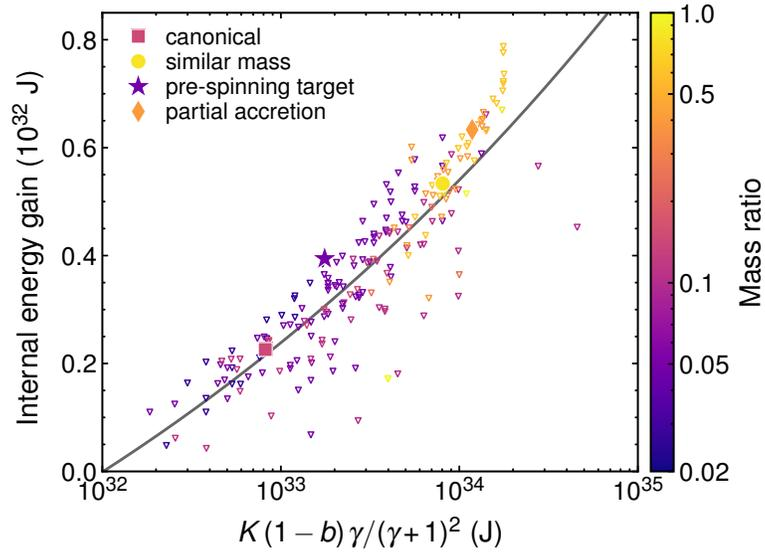
**Figure S1.** Internal energy gain of the system at 24 hours after the impact as a function of modified kinetic energy. The grey line is the scaling relationship given in equation S1. The colours of the points indicate the ratio of projectile to target mass. The four example impacts shown throughout this work are indicated by unique symbols.
